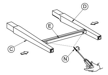
STEP 5: Using the Allen Key to tighten all bolts.
